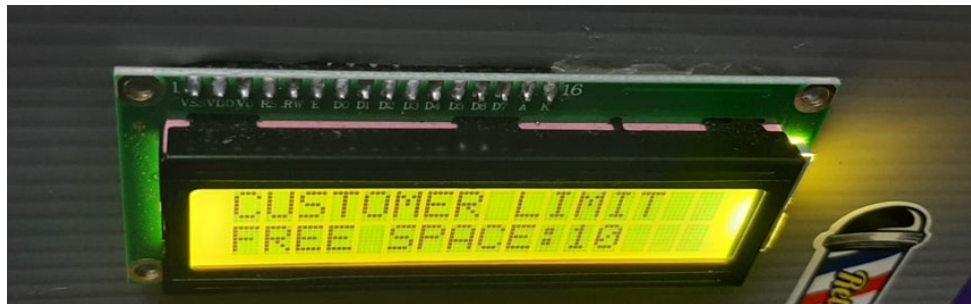
Figure 7. The LCD display of space available for customer to enter the shop or place.
